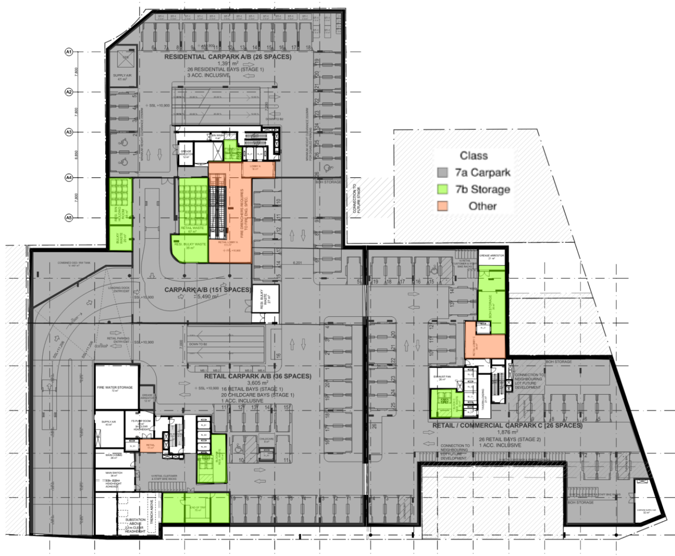
Figure 2: Basement 1 layout (indicative of all basement levels)
