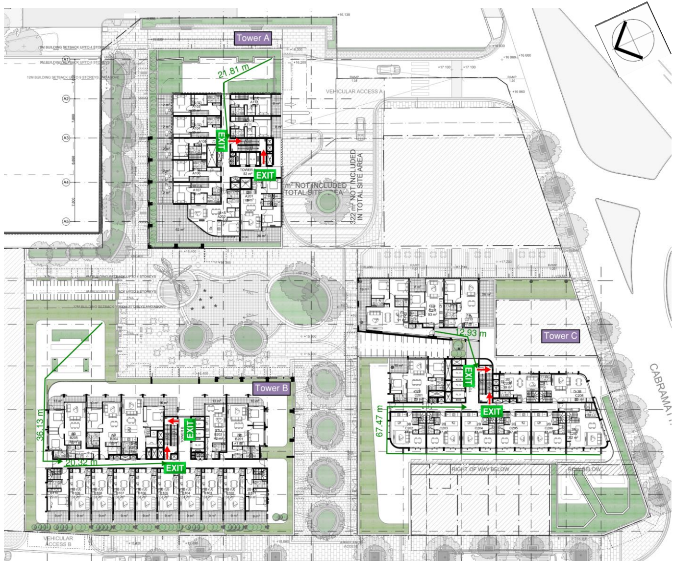
Figure 10: Egress and exits arrangement – level 2 (indicative of all residential levels except topmost)
